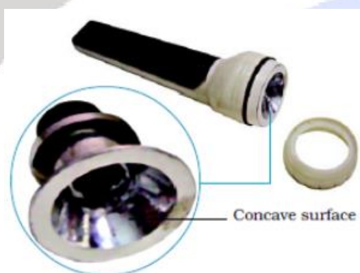
Figure 13: Concave Mirror Used in Torch
