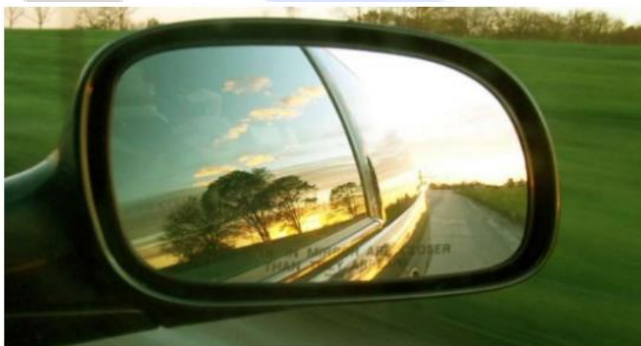
Figure 14: Convex Mirror used in a Rearview Mirror
