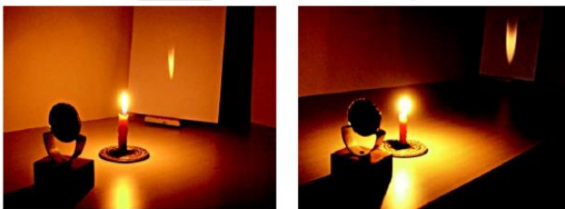
Figure 11: Formation of Real Image by Concave Mirror
